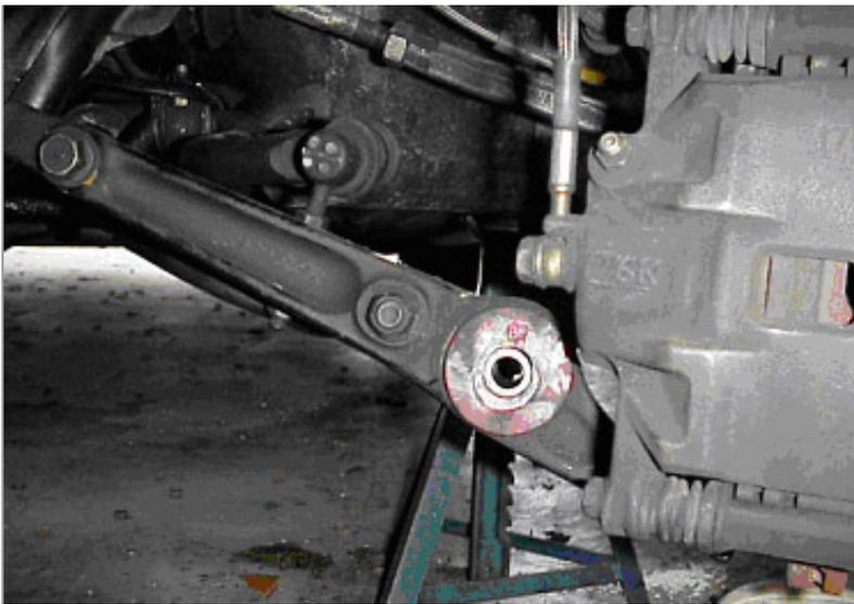
The bushing in this lower control arm shows the result of using incorrect suspension geometry in a traction bar. As one can clearly see, there is a severe tear all the way around the bushing.
