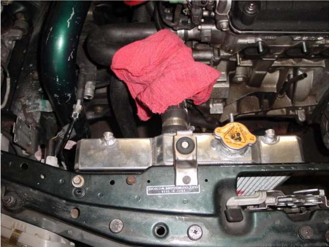
Figure 6. Installed radiator top view
