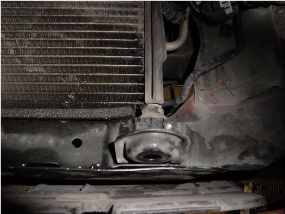
Figure 1. Radiator tab spot weld drilled.
