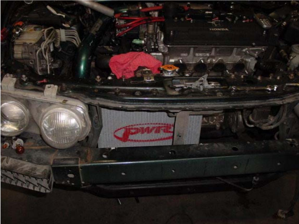
Figure 5. Installed radiator front view
