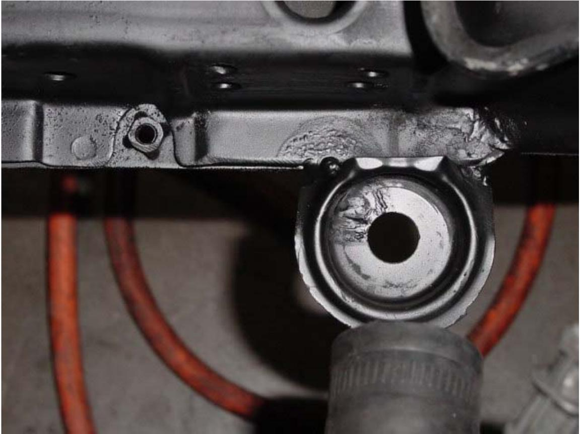
Figure 4. Welded lower radiator mounting tab
