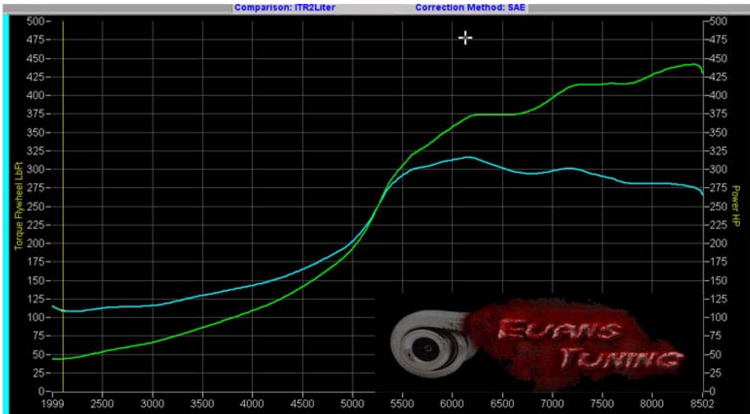
Figure 7. T3/T67 @ 16 psi with pump gas.
