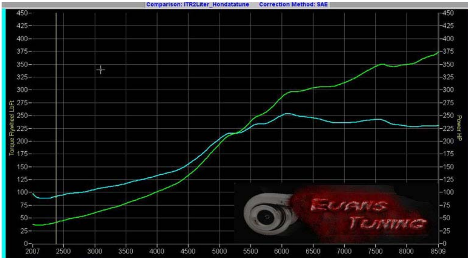
Figure 14. T3/T67 @ 14 psi on pump gas.
