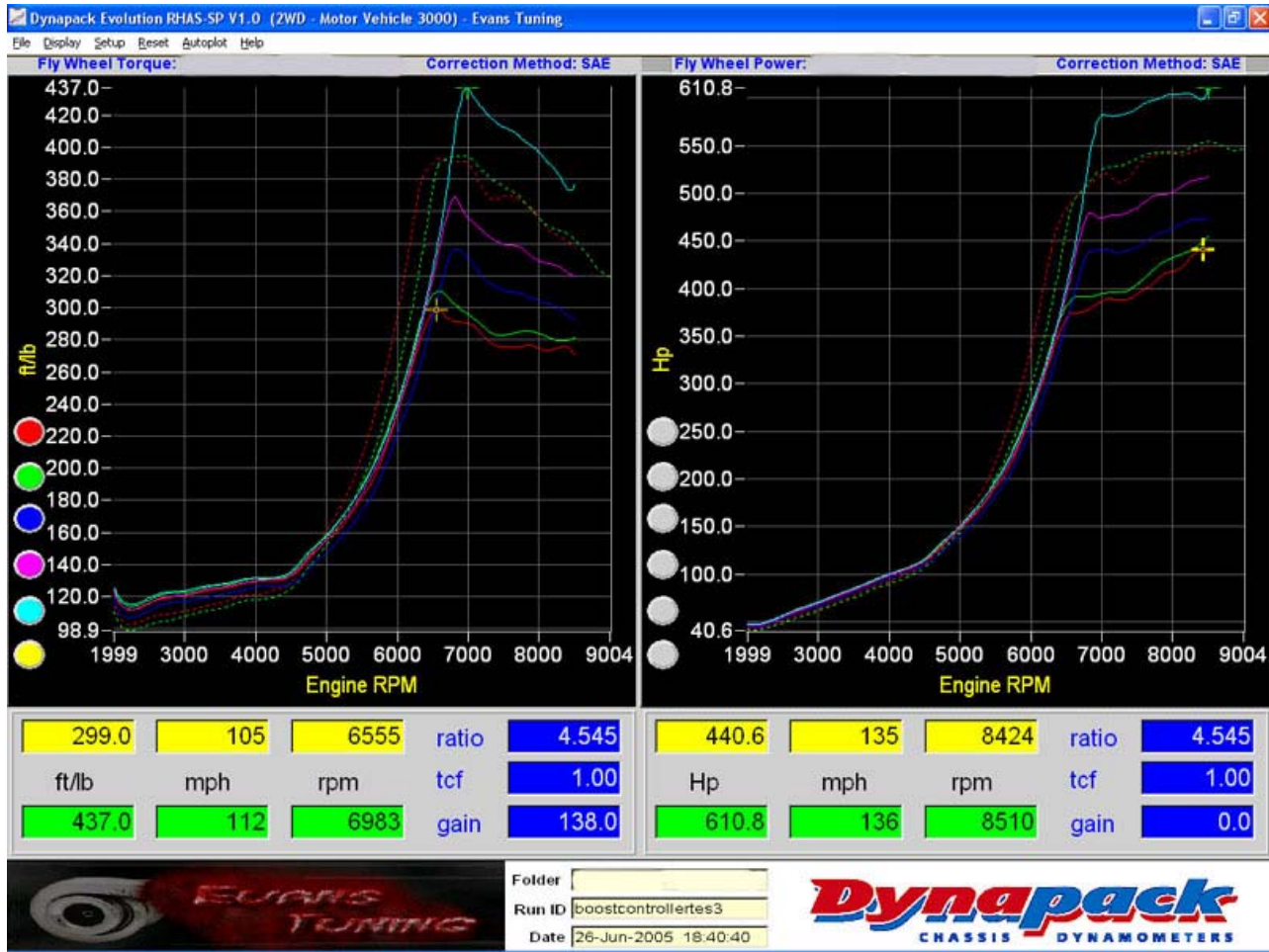
Figure 1. Full Race T3/T67 H.O. turbo @ 28psi with race gas.
