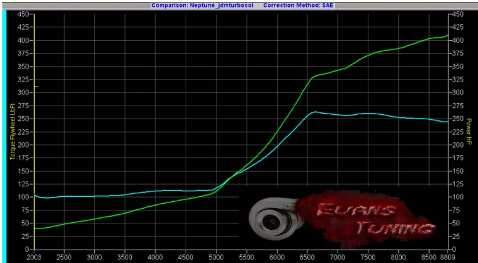
Figure 2. T3/T67 H.O. @ 15 psi with pump gas.
