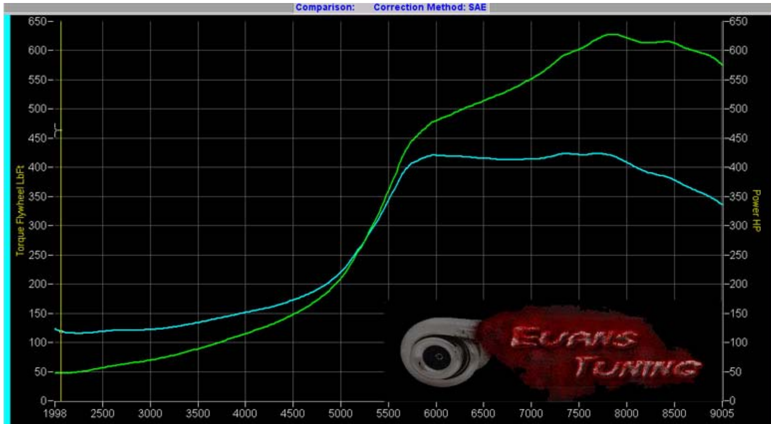
Figure 12. T3/60-1 @ 25 psi on race gas blend fuel.
