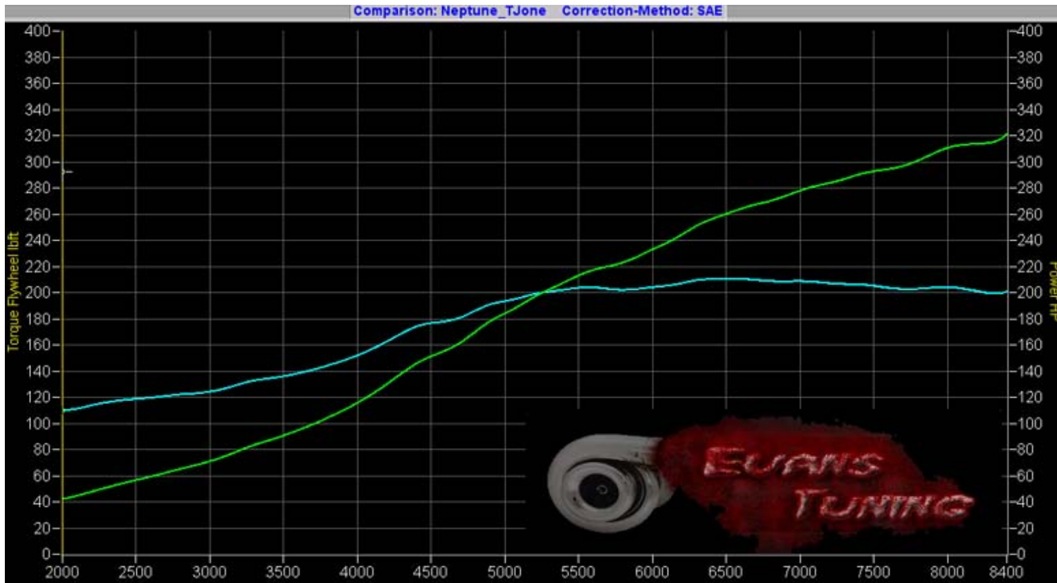
Figure 10. T3/T04E 60 trim @ 9 psi on pump gas.
