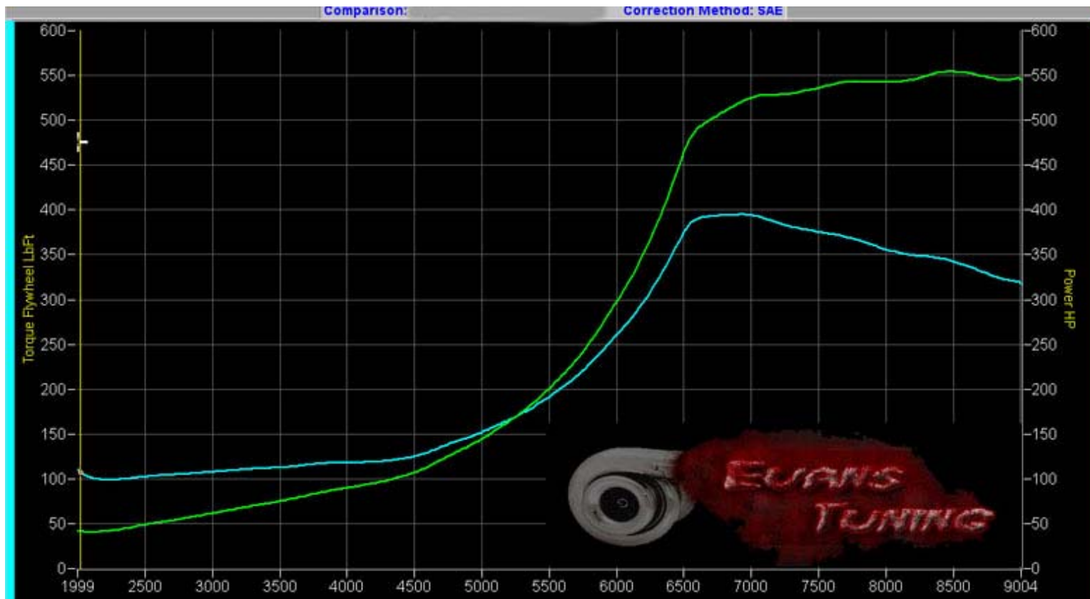
Figure 9. T3/T67 H.O. @ 24 psi on race gas blend fuel.
