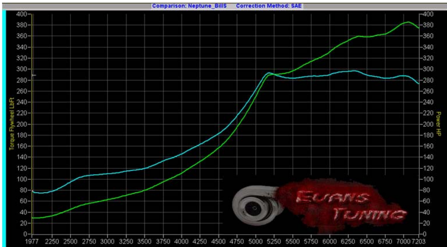
Figure 4. T3/T67 turbo @ 15 psi with pump gas.
