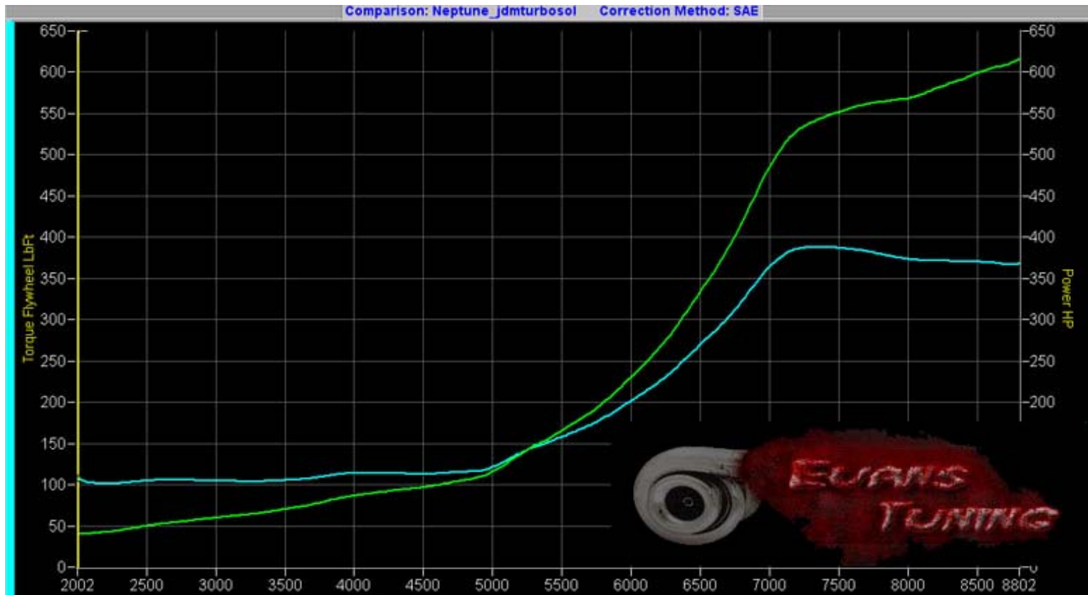
Figure 3. T3/T67 H.O. @ 30 psi with race gas.
