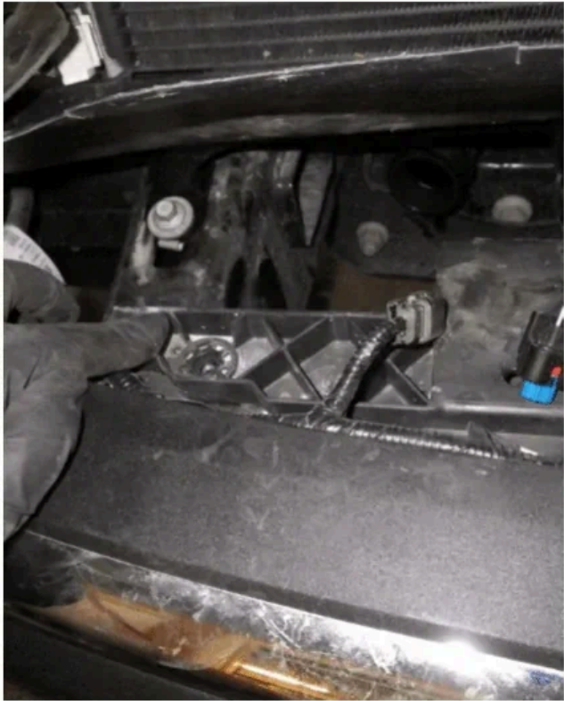
16a. Start with the shutters, separate the rubber cover and unplug the shutters motor
