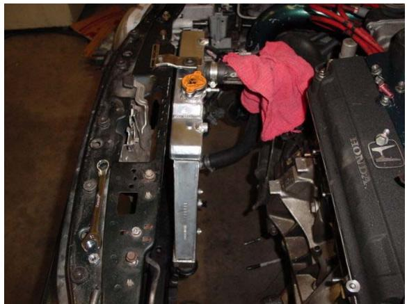
Figure 7. Installed radiator side view
