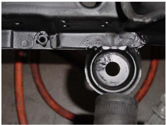
Figure 4. Welded lower radiator mounting tab
