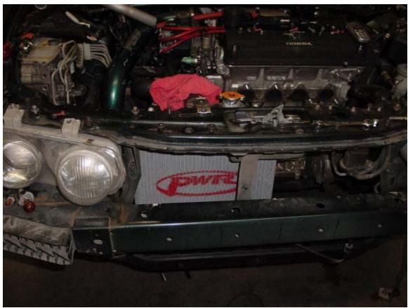
Figure 5. Installed radiator front view
