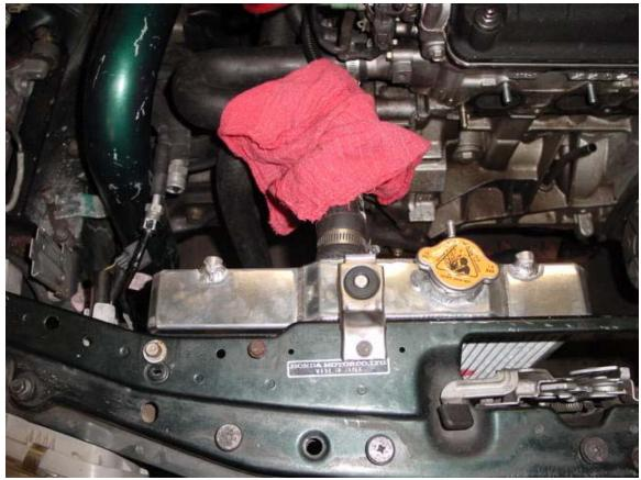
Figure 6. Installed radiator top view
