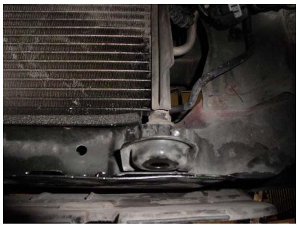
Figure 1. Radiator tab spot weld drilled.
