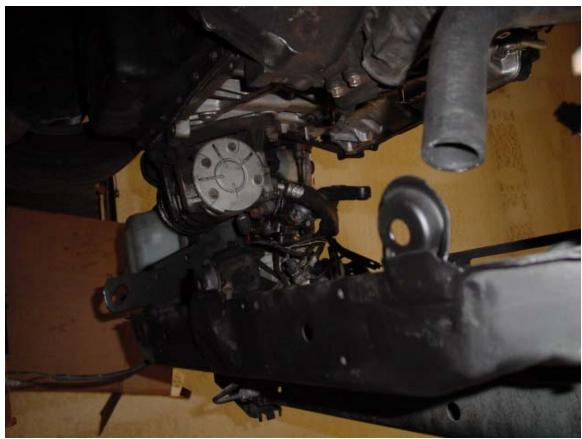
Figure 5. Welded lower radiator mouting tab
