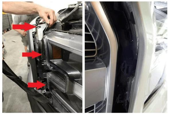
**Step 8.** Remove x2 8mm bolts from each lower corner of the grill using an extension and 8mm socket.
