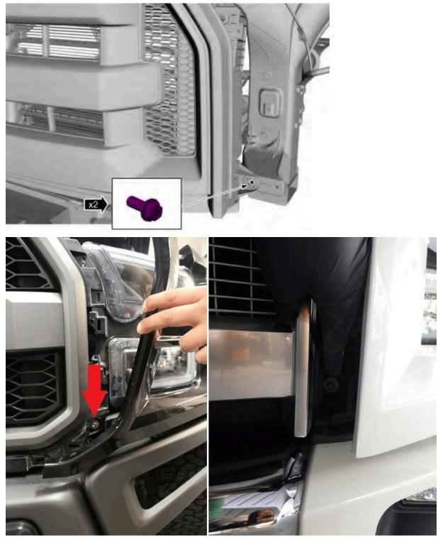
**Step 9.** Find a safe place to set the Grille. Carefully lift and remove grille assembly out of the vehicle. Avoid scratches / scrapes.
