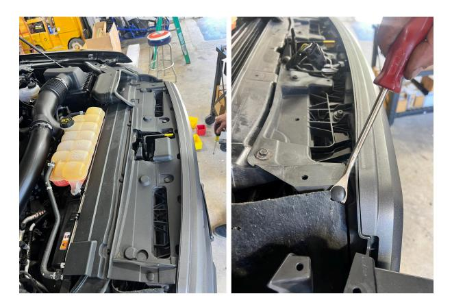
2021+ trucks have 2 more trim clips on the corner of the core support, 2 small 7mm bolts on each of the passenger/driver side fender liners, and a corner lamp that needs unplugged.
