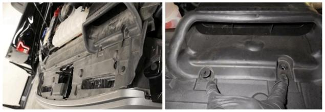
Remove (7) clips holding the radiator air deflector. Gently pry the center up until it unlocks, then pull on the larger round base to remove.
