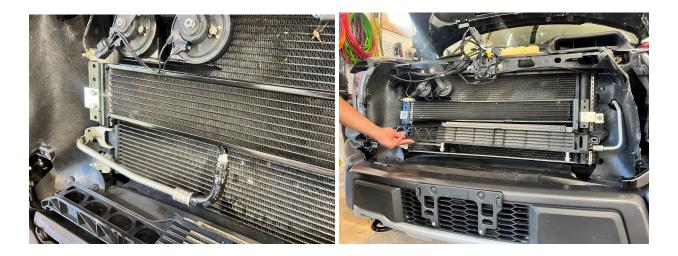
**Step 15.** Reinstalling grille: Double check that everything is tight, secure and plugged in. Reinstall grille assembly in reverse order of disassembly. Be sure to plug in all connections by the hood latch. Go over all work, ensure there is nothing overtightened or loose/disconnected before reinstalling grille, headlight surrounds, and plastic front cover pieces.
