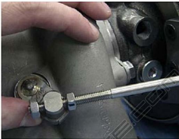
Figure 83: Holding Valve Closed with Nuts Loosened
