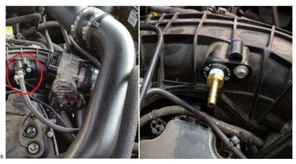
**6.** Using a small pick tool or screw driver, remove the spring and check valve from the PCV. Now is a good time to use a drill bit and remove this "step" to enlarge the opening. (Drilling is not mandatory). Reinstall gutted-PCV valve in RHS valve cover.
