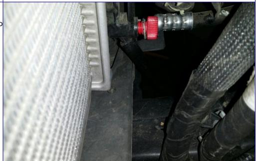
Ensure hose will remain in drain pan and allow coolant to drain, you can continue with work on radiator while draining
