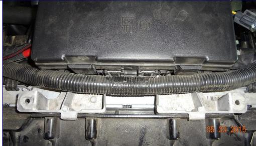
Separate chassis harness from plastic radiator shroud Once harness is removed move fusebox on top of throttle body
