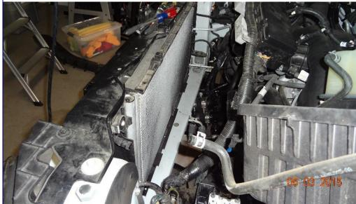
If using Raptor fan skip to next step, if using F150 OEM begin trimming shroud to fit new radiator
