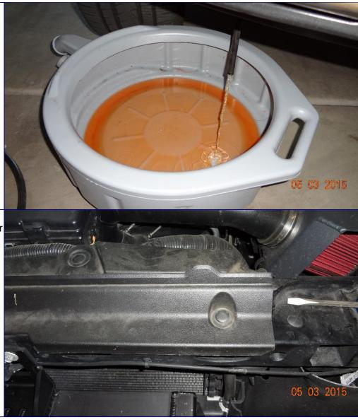
Carefully remove 4 clips from upper radiator cover Remove upper cover and set aside
