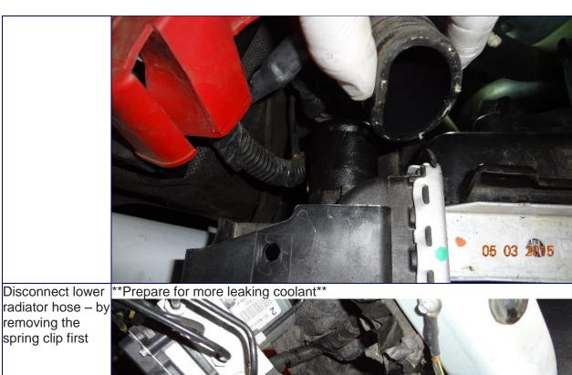
radiator hose – by removing the spring clip first
