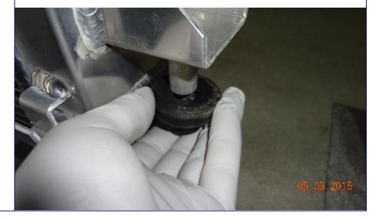
Install radiator, driver's corner first then wiggle the passenger side into place Tilt radiator forwards to slip AC condenser into place Put radiator/AC
