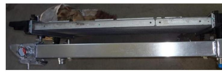
In order to properly cool this engine, we use an oversize radiator. Converting to this style radiator with traditional cap requires removing the tank from the airbox and trimming the fan shroud top lip from the radiator. We also include the option to use a traditional radiator cap and overflow tank – similar to SVT Raptor's cooling system for extreme off-road or big turbo / high power applications.
