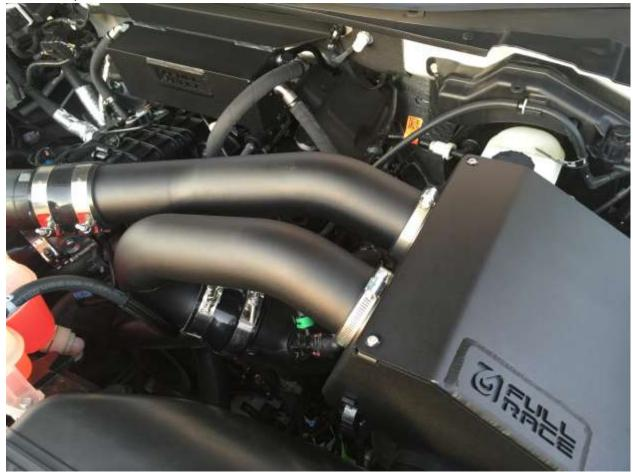
**14.** Inspect the install. Check all hose clamps for tightness, without being overtightened. Check sensor installation and plug. Check air box clips. If everything checks out - connect battery, start engine.
