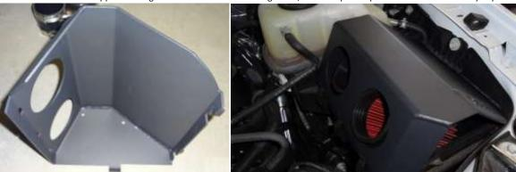
**10.** Align the **rear** intake pipe/filter/clamp. Inspect coupler and filter/housing alignment, then tighten. This rear filter can be tricky to align on 2011-2014. It is easier on 2015+.
