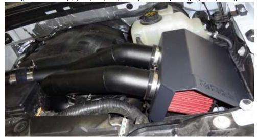
12. Install intake sensor, and plug in. 2011 in front pipe, 2012-2016 in rear pipe.
