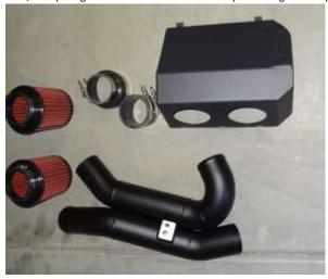
7. Place the 3" straight coupler/clamps on the passenger side and 4" -> 3" transition "step coupler"/clamps on driver side.
