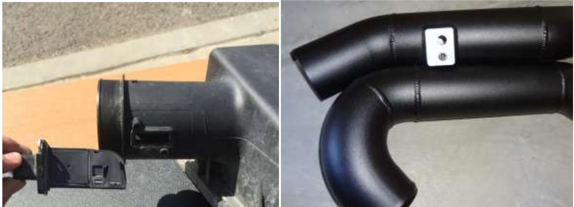
3. Loosen clamps #7, #5, #6, #8 (optional). Unclip lower airbox #1. Remove filter element #4, Merge pipe #9 and upper airbox #3.
