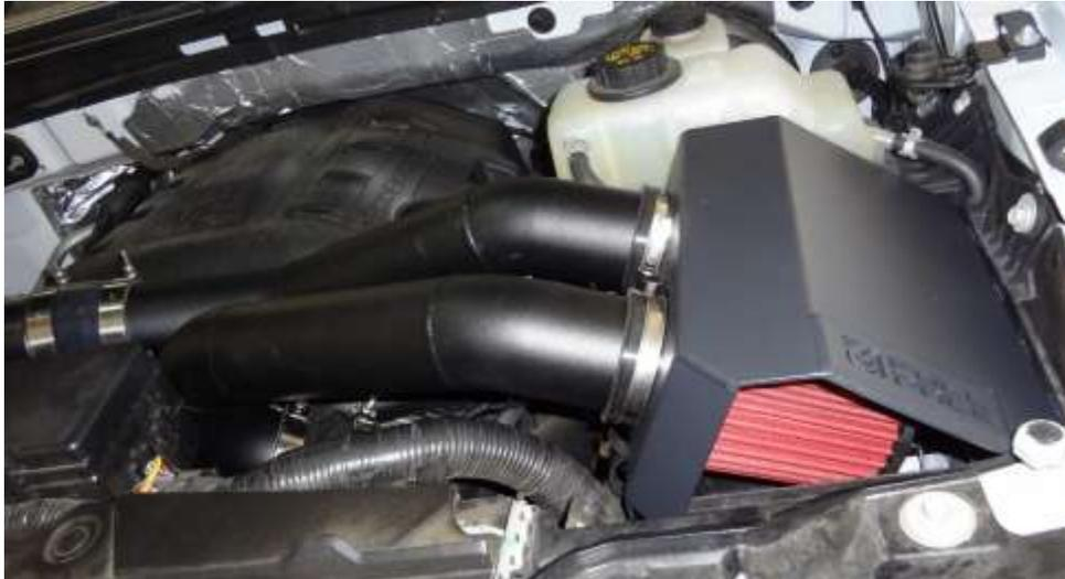
12. Install intake sensor, and plug in. 2011 in front pipe, 2012-2016 in rear pipe.
