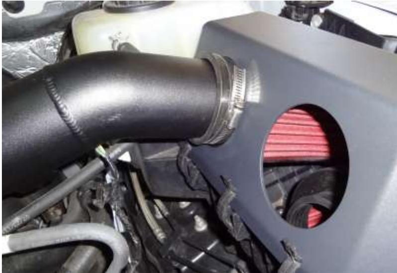
11. Align the **front** intake pipe/filter/clamp. Inspect coupler and filter/housing alignment, then tighten.
