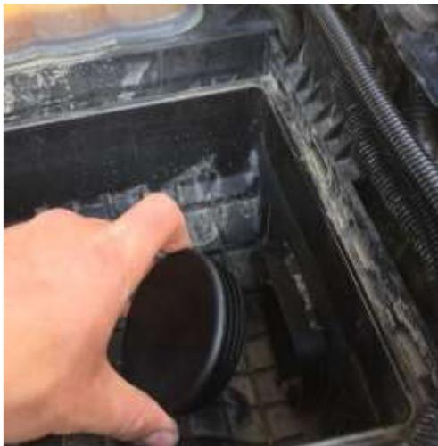
9. Install the airfilter upper housing with air filter elements. Align tabs, lock in clips. Keep airfilter elements loosely in position.
