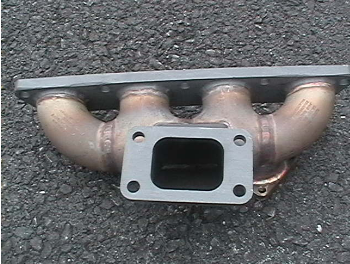
Figure 2. Fabricated log manifold, bottom view.
