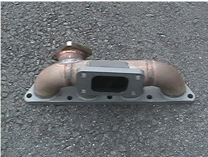
Figure 3. Fabricated log manifold, front view.
