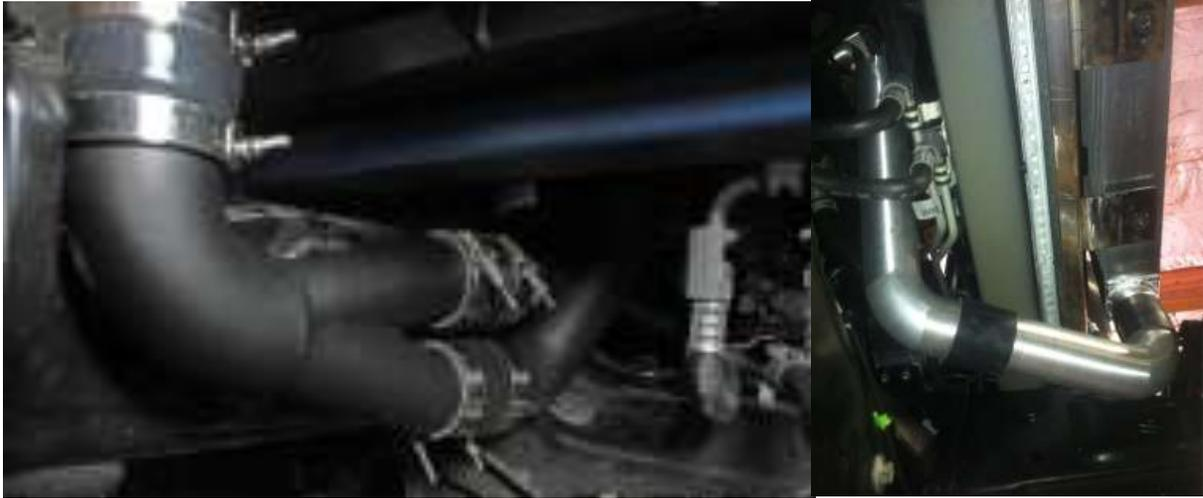
9. Now that the mounting beam is tightened and the Y-pipe is loosely in place - we can install the intercooler. NOTE: the hood latch should remain in the stock location, sandwiched between the headlight/radiator support and the intercooler's upper mount:
