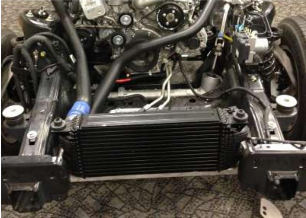
7. Begin installing the Intercooler Mounting Beam, use the 10mm socket and long extension to firmly tighten in place:
