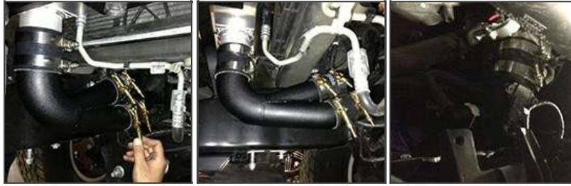
14. Test fit the Grille for clearance. Make sure there is nothing rubbing.
