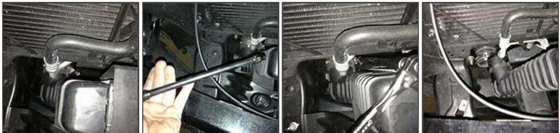
6. Unbolt the lower mounting bracket - to allow the stock CAC to drop out the bottom. **Removal of front spoiler/air dam may be required to aide in CAC removal.** Also remove the factory hotside couplers. After this step the stock CAC and its components are out of the vehicle and we can begin installing
