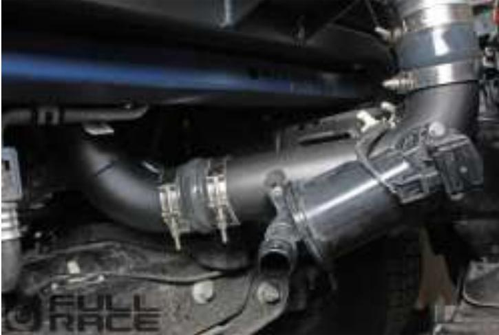
If Full-Race Catch can AND external BOV are used, the PCV delete location is ideal for BOV vacuum signal.
