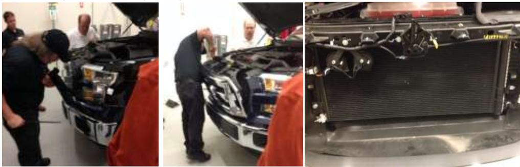
2. Remove Shutter Assembly from Grille. Leave plug disconnected (it will not throw a code). You will need to gently cut the plastic center piece away.
