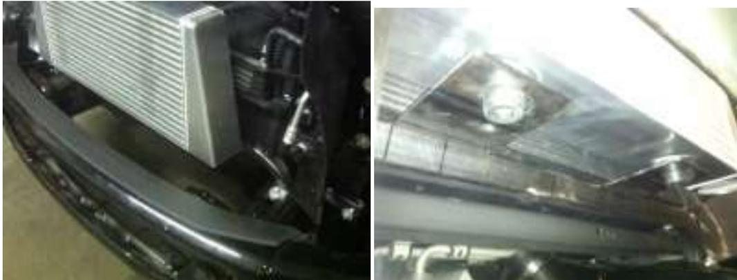
8. Install the (2) Full-Race 2.5" straight couplers on the hot pipes and get the Y-pipe oriented (it helps to use soapy dish water in a squirt bottle when sliding these on). Keep the clamps loose - do not tighten yet.
