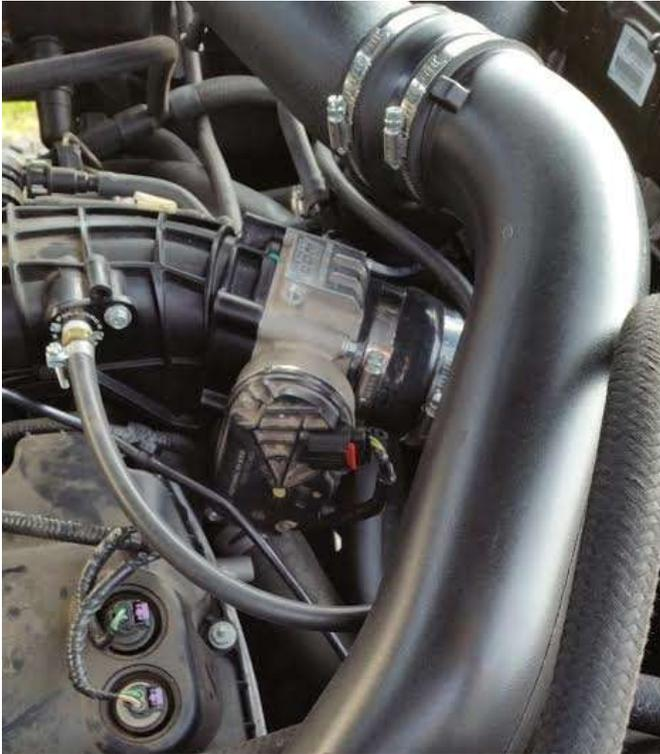
13. All pipes and couplers should be in place, ready for the clamps to be tightened down. Align and orient the clamps as shown, then tighten down. **Do not go crazy and overtighten, it can crush the tube or cut the silicone coupler:**
