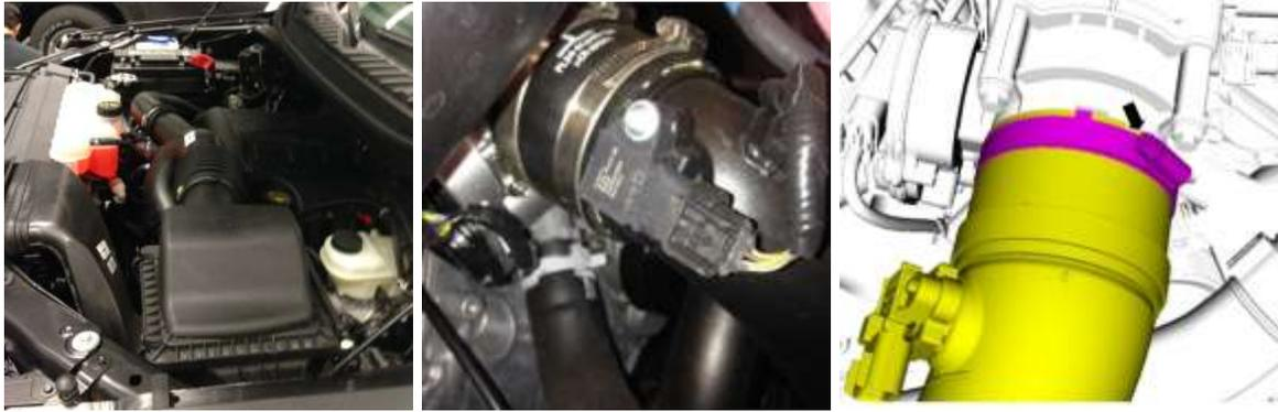
4. With the intake out of the way, unplug the MAP sensor and disconnect the PCV hose (located just before the throttle-body). Loosen the Throttle-Body (cold-side) hose clamp to release the coupler, then use a small flathead screwdriver (or your fingers) to free the spring clip <#4 in the photo>. Remove charge pipe from engine bay. Unbolt E-BOV from CAC if it will be retained:
