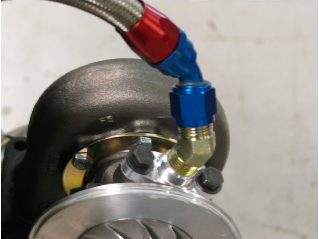
Figure 1. CHRA oil drain fittings.
